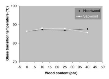
Figure 3. Change in glass transition temperature as a function of wood content.
